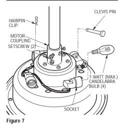
☐ **15.** Tighten the two upper setscrews (Figure 7) securely while pulling up on the downrod.
